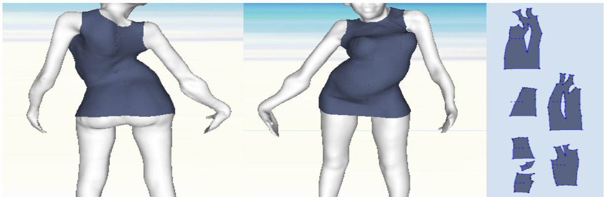
Figure 1: Customized garment design for scoliosis patients using CAD tools (interactions between 3D virtual garment fitting and 2D garment patterns generation)
